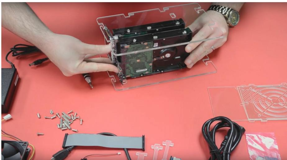
**Assembling an ODROID XU4 CloudShell 2 NAS Unit**
